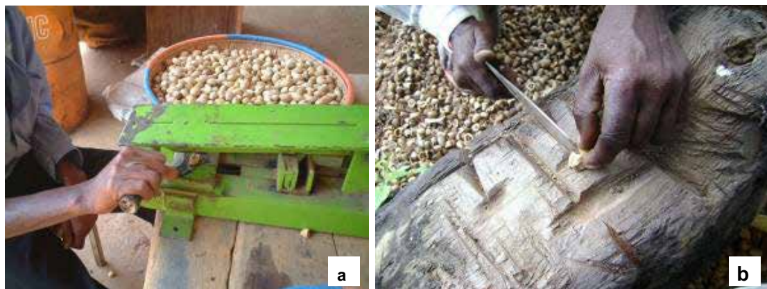
Plate 3.3: Extraction of Melia seeds from nuts using: (a) a Melia nut cracker and (b) knife
